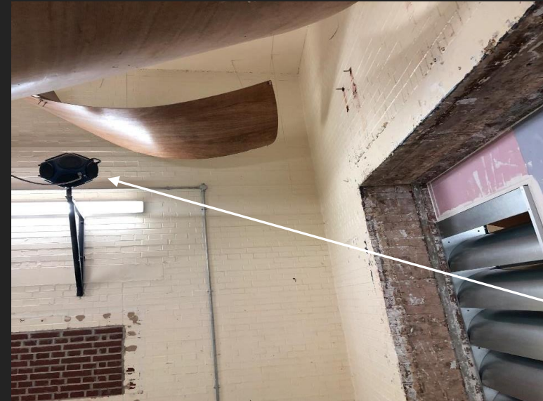
Omni directional Loudspeaker used to excite the room
